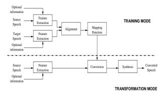
Figure 1: VC system block diagram
