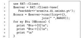
The first line imports the NAT::Client module, which includes the API for querying NatServer. The second line creates a new client. Here we can specify the remote host where the queries will be send, or the local path for a local corpora we want to query. In this case, we change the client creation code to:
